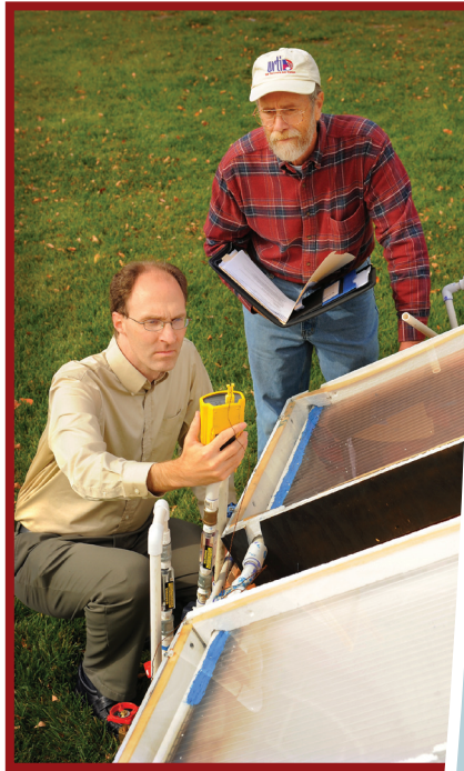
Chemical engineering associate professor Kevin Dahm (kneeling left) and Helios Products, LLC, founder Neal Cramer read a temperature indicator for a prototype solar panel that was built by a Rowan clinic team.
