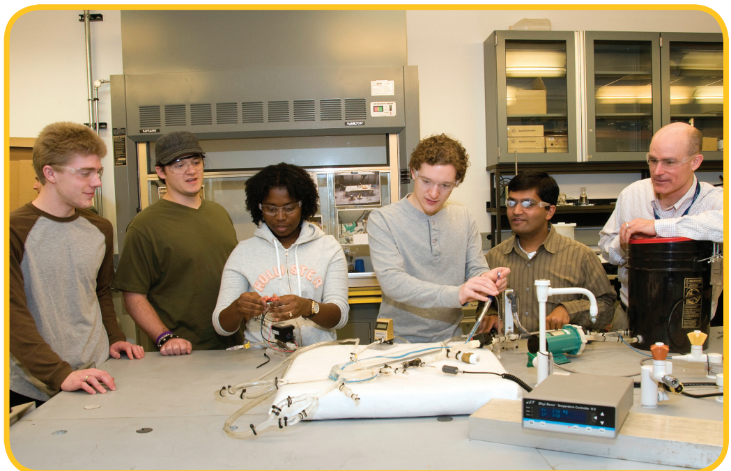
Mechanical engineering students (l-r) Chris Rakus , Larry Greco , Casey Oware , John Zacharkow , and Dhaval Naik work with Dr. Thomas Merrill on their mock circulatory system, which is designed to test a new catheter capable of cooling the heart nearly 10 times faster than present technology.
