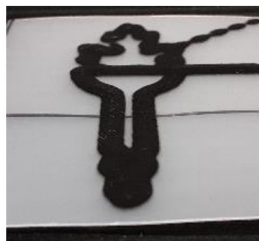
Cold Sprayed Polymer with High Deposition Efficiency
