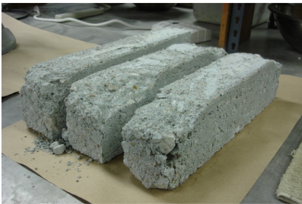
Concrete can deteriorate due to freezing
