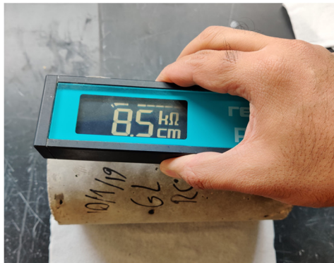
AASHTO T358 Surface Resistivity Test
