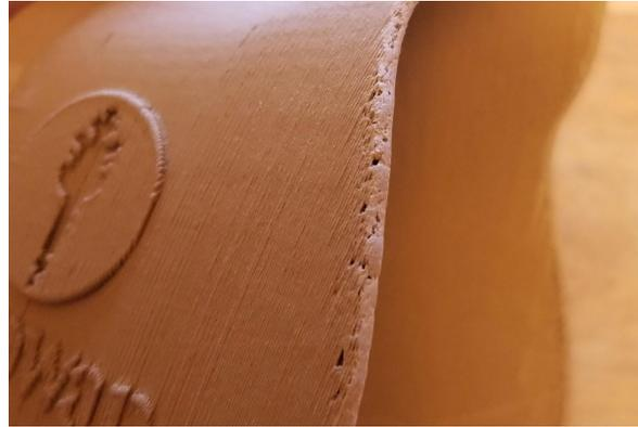
Small superficial damage do not affect the structural integrity of the print.
