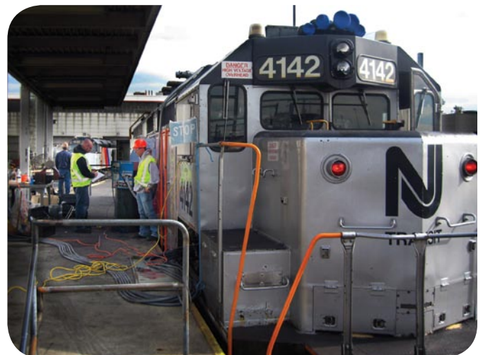
Engineering professors and students are measuring emissions from diesel locomotives operating on different fuel blends.
